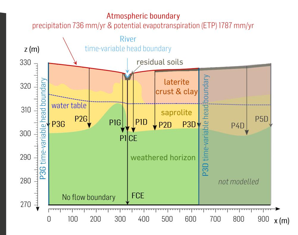
The 630 m long 2D modelled profile with the 4 formations considered, the boundary conditions and the location of the observation wells
