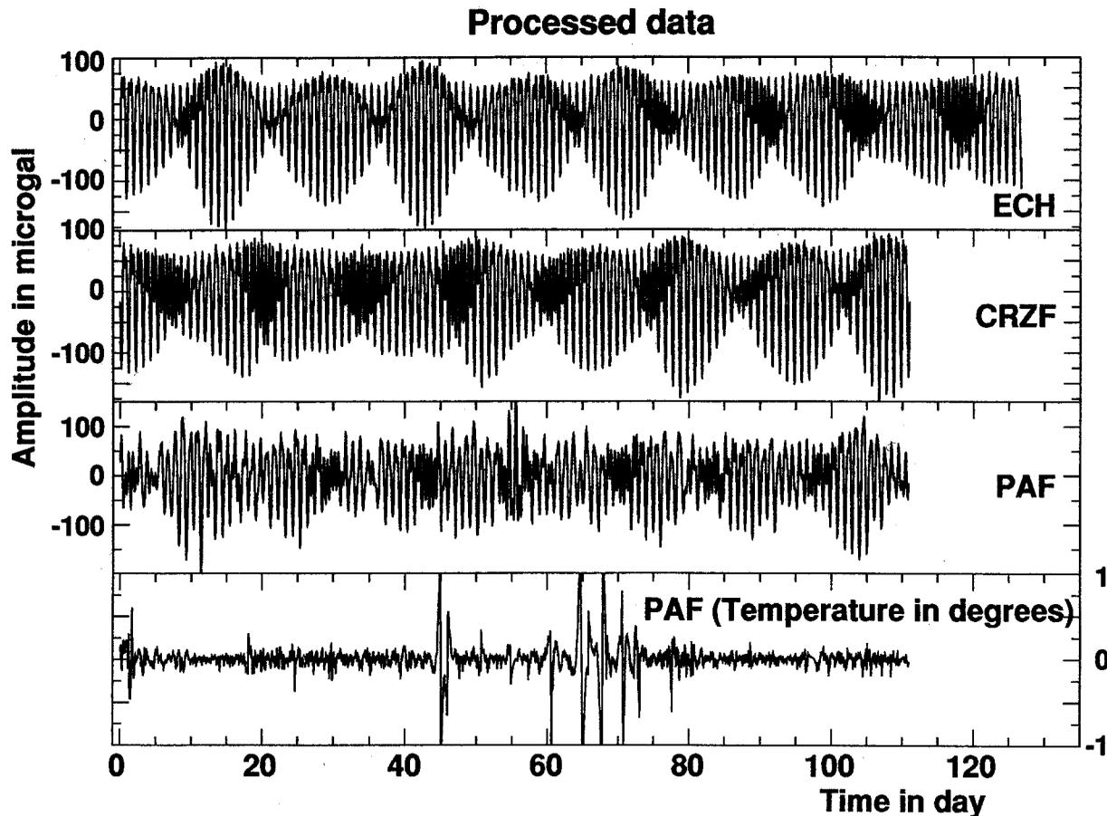
Fig. 6. Processed data at ECH, CRZF and PAF with the temperature at PAF. The duration is about 3 months.
