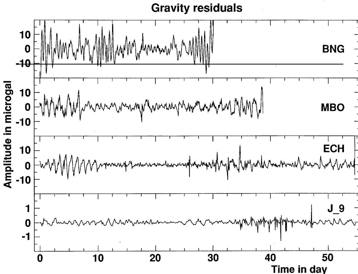
Fig. 9. Tidal residuals at BNG, MBO, ECH and J-9. The scale factor for J-9 is 10 times smaller than the others.
