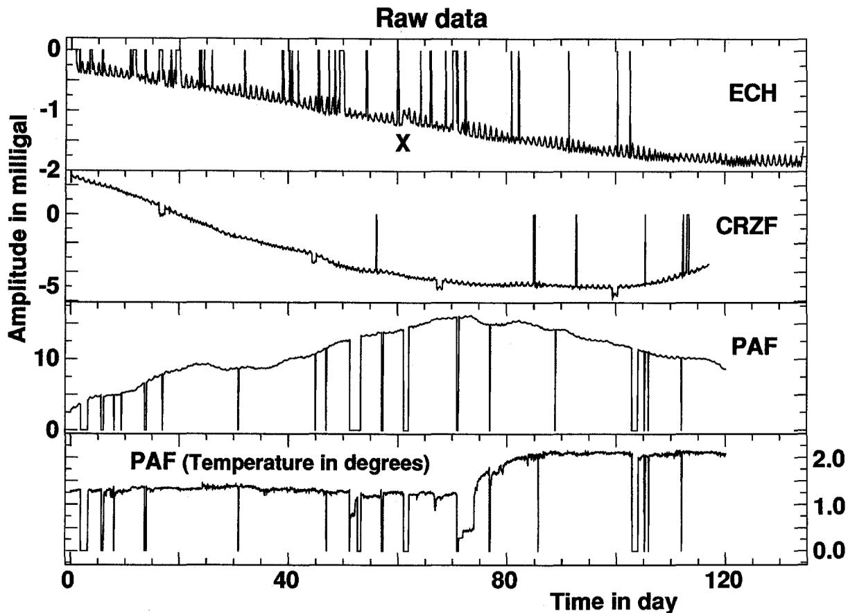
Fig. 3. Raw data at ECH, CRZF and PAF with temperature at PAF. These signals are plotted before interpolating the gaps. The duration is about 3 months. On ECH, the disturbance marked X should be noted.
