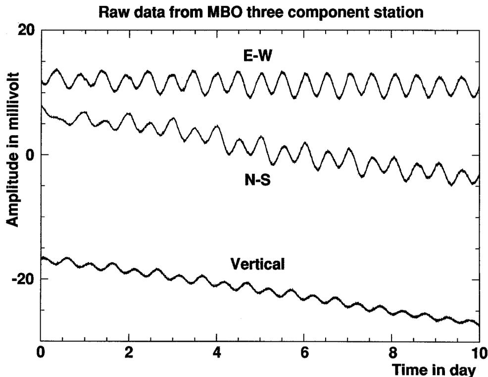
Fig. 4. Raw data from MBO three-component station. The tides are clearly visible on both vertical and horizontal components.
