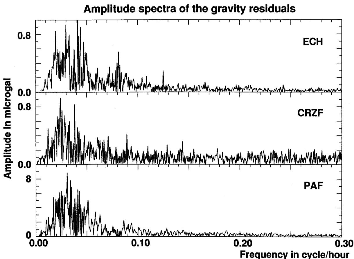
Fig. 12. Comparison between the spectra of tidal residuals at ECH, CRZF and PAF. The corresponding time duration is close to 120 days. The short-period high-level noise at PAF was possibly induced by adverse meteorological conditions.
