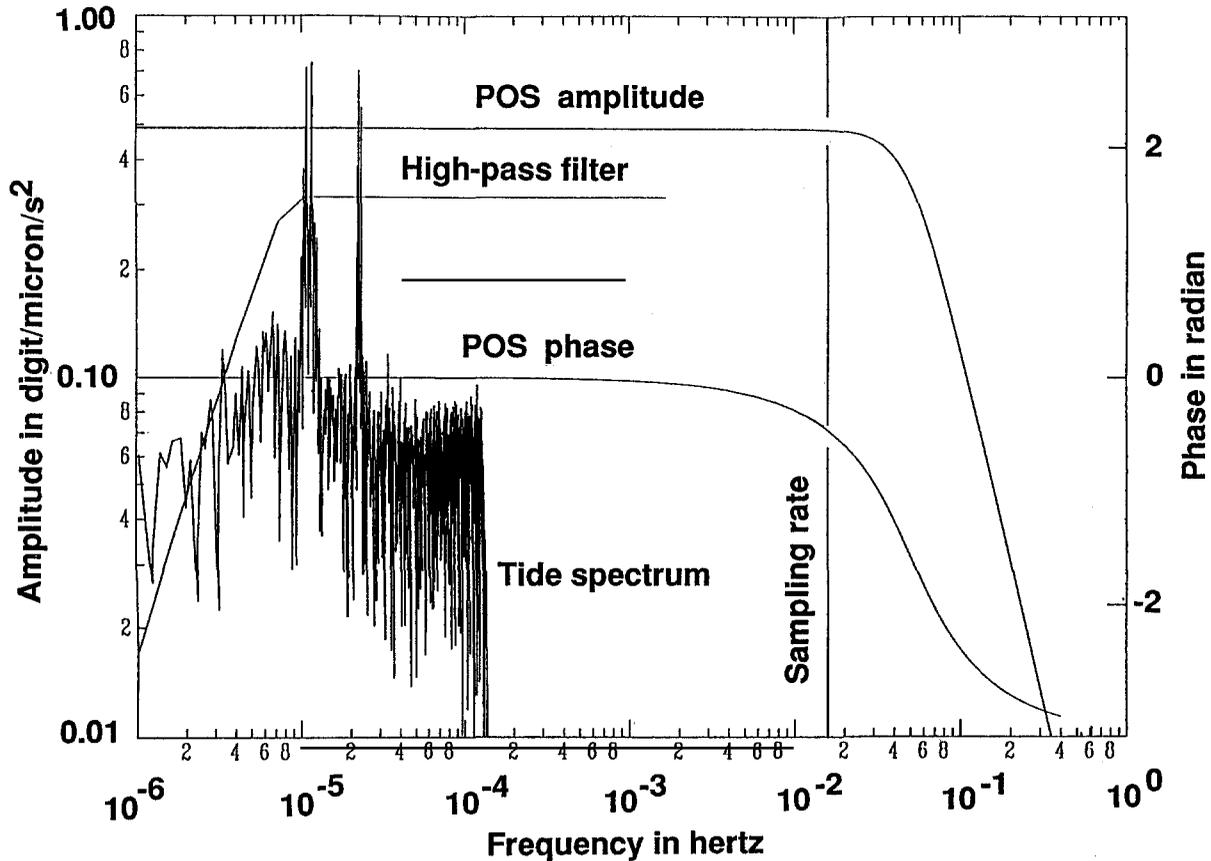
Fig. 1. Bandwidth of POS (amplitude and phase) and convolution high-pass filter with cut-off frequency at 1/46 h. A tidal spectrum is also plotted.
