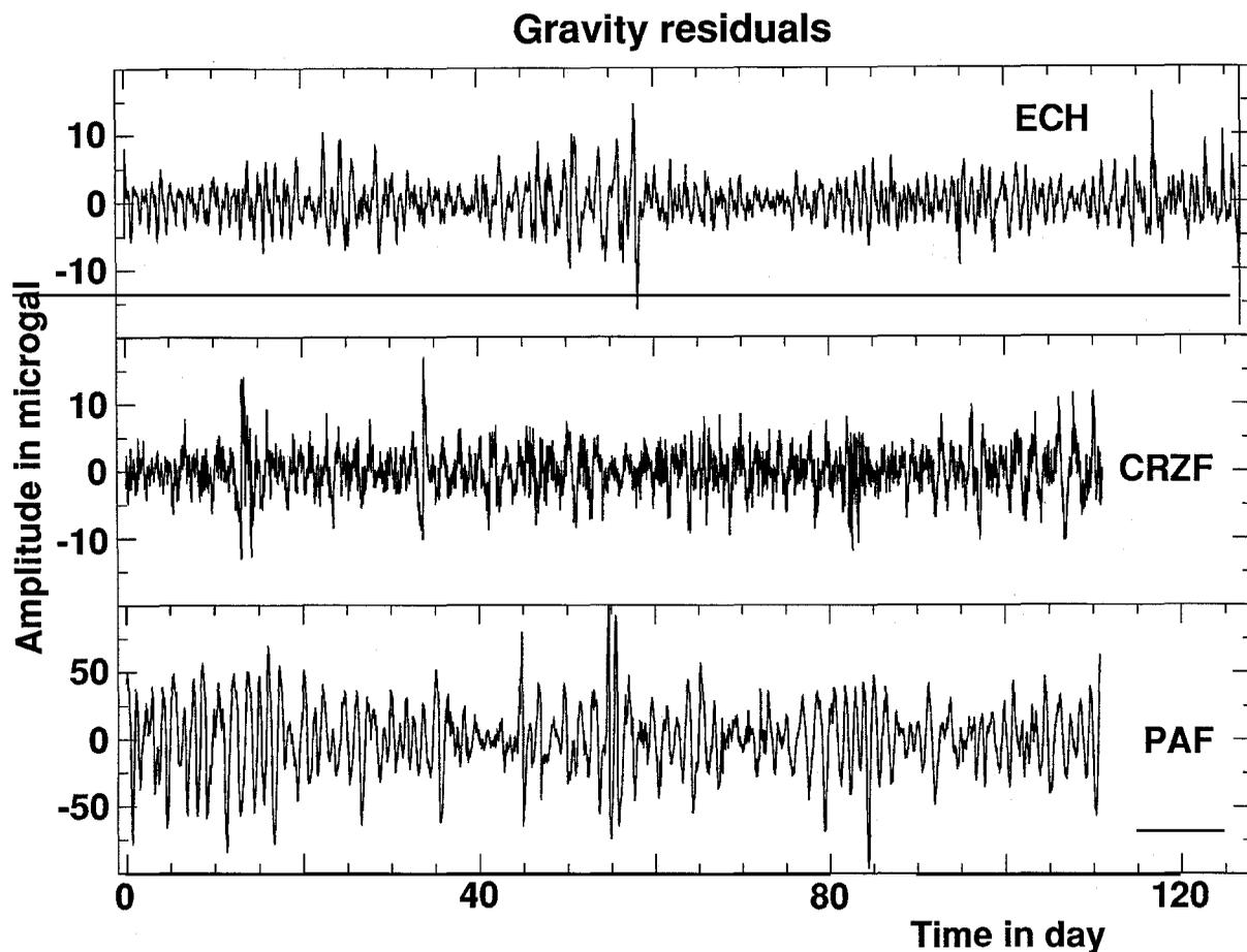
Fig. 10. Tidal residuals at ECH, CRZF and PAF. The duration is about 120 days. The scale for PAF is five times larger than the others.
