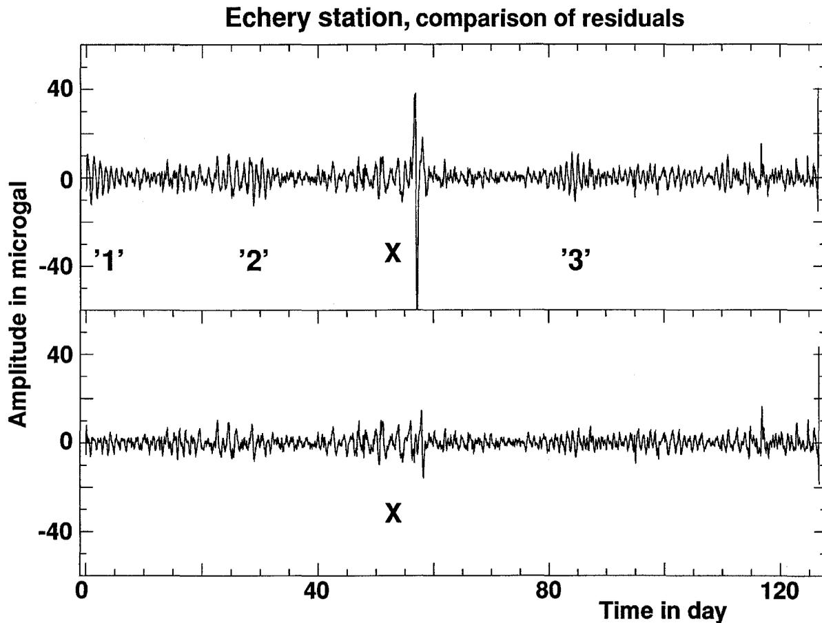
Fig. 14. The upper signal is the residual signal at ECH without correcting for the disturbance X in Fig. 3 before the tidal fit. The lower curve shows the residuals after correction. (Note the reduction of the noise peak close to the area X and the attenuation of the noisy segments marked '1', '2' and '3'.)
