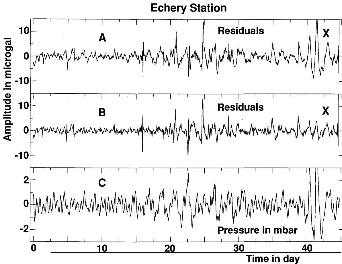
Fig. 13. Pressure influence at ECH: the signal A shows the gravity residuals without any correction of the pressure, C, and the signal B is after pressure correction. The noise reduction is very clear at the end of the signal (marked X).
