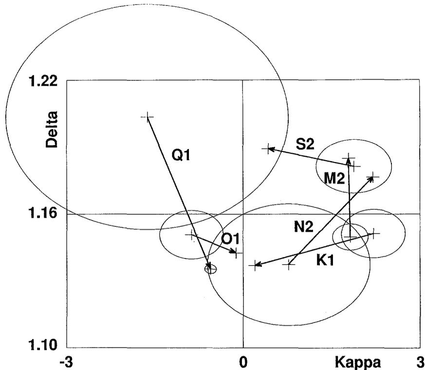
Fig. 8. Comparison of the results obtained at ECH (55 days) and at J-9 (55 days). The ellipses represent the r.m.s. errors on gravimetric amplitude and phase factors. The arrows start at the location of the results for ECH and end at the location of the results for J-9.
