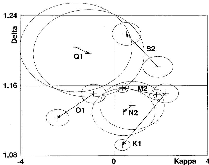
Fig. 7. Comparison between analysis of two sets of data at ECH, the durations being 55 and 127 days, respectively. The ellipses show the r.m.s. errors on the gravimetric amplitude and phase factors. The arrows start at the location of the results for the shorter duration (55 days) and end at the location of the results for the longer duration (127 days).
