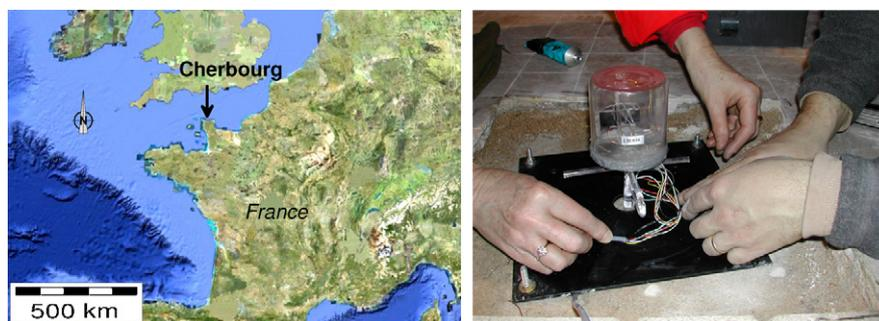
Fig. 1. Site location and installation of a Blum Pendulum in the “Souterrain du Roule” at Cherbourg (France).
