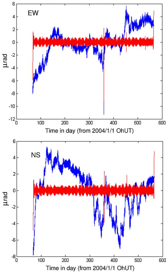
Fig. 2. EW and NS raw and band-pass filtered tilt records at Cherbourg.
