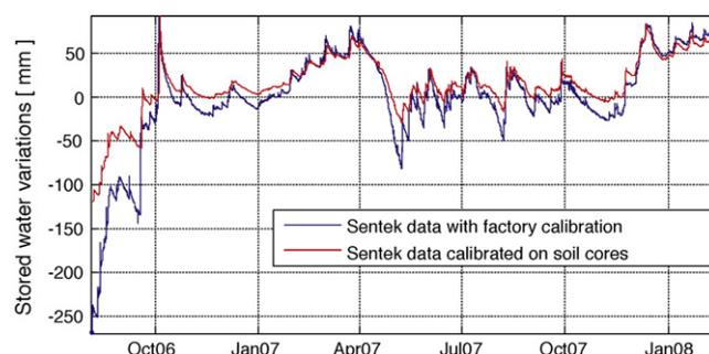
Fig. 2. Stored water variations of the entire soil thickness above the gravimeter before (blue) and after (red) calibration of the probes on soil cores. Note the highly non-linear calibration. (For interpretation of the references to colour in this figure legend, the reader is referred to the web version of the article.)
