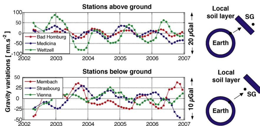
Fig. 1. Monthly gravity residuals observed at several GGP stations after reduction of tides, polar motion and atmospheric contribution. Stations are classified with respect to the relative position of the gravimeter with the local soil layer, above ground or below ground. Adapted from Crossley et al. (2006). (Colour figure can be viewed in the online issue.)
