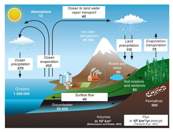
Figure 1.1 – Water cycle and the global mean storage  $(10^3 \text{ km}^3)$  and annual fluxes  $(10^3 \text{ km}^3.\text{yr}^{-1})$ . Adapted from Shiklomanov and Rodda (2003) and Trenberth *et al.* (2007).
