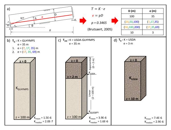
**Figure 3.4** — Aquifer scheme used on transmissivity estimation, assuming a linear, unconfined, homogeneous isotropic aquifer. Transmissivity is given by the product of a) saturated depth (e) and three hydraulic conductivity data (K): b) using GLHYMPS data, c) combining USDA and GLHYMPS data, and d) using USDA data. WT = water table, T = transmissivity, K = hydraulic conductivity, e = saturated thickness, p = linearization constant, D = aquifer depth, B = aquifer length,  $\theta$  = slope.
