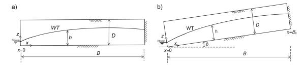
Figure 3.1 – Aquifer scheme proposed by a) Brutsaert (2005) and b) Zecharias and Brutsaert (1988). WT = water table; D = aquifer depth; B = aquifer length; h = water table elevation;  $\theta$  = aquifer slope; z and x are the vertical and horizontal axes, respectively.
